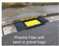
Each Piranha Filter comes with a pre-cut back-block for grates with curb openings. Simply fold in half and put under the Piranha Filter prior to installation. The attached Velcro will hold the back-block in place. The back-block is 6" high.
